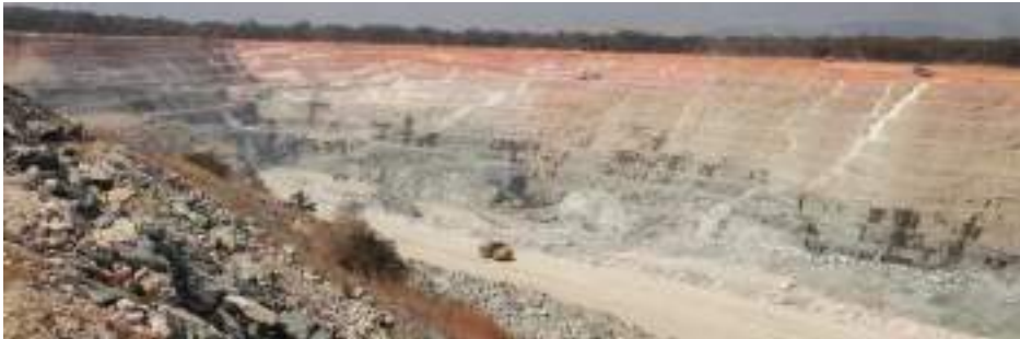
The pit depth at Chama is now down to around 110m from surface, with a west to east strike length of approximately 900m
