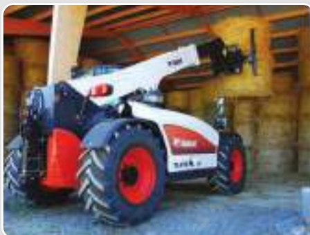
The TL470HF telescopic handler offers higher horsepower engine and a 190l/min load sensing hydraulic pump
