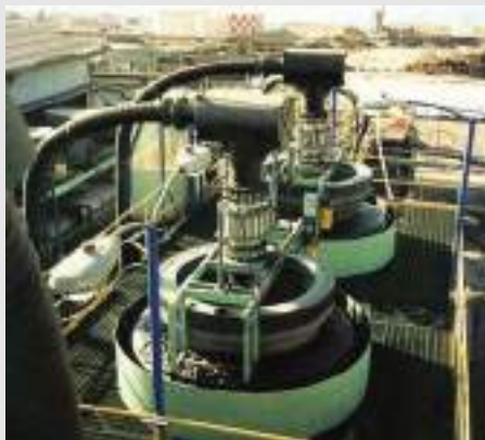
Pneufлот cells are simple in design, with a high yield of froth product
