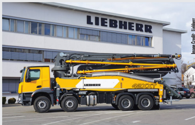
A truck mounted with the concrete pump 42 XXT.
