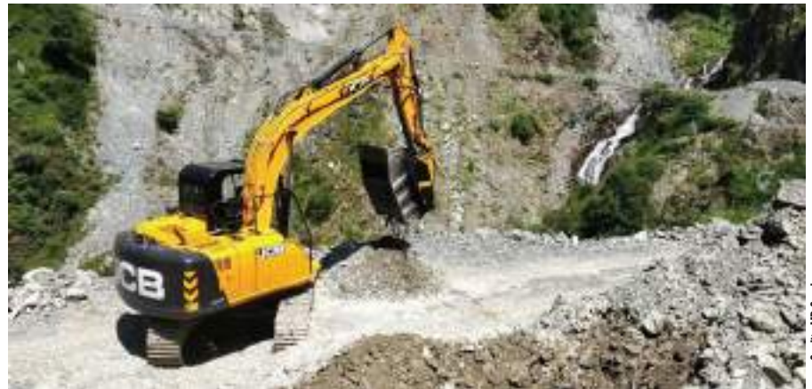
Recycling river bed material in India with the BF70.2 crusher bucket.
