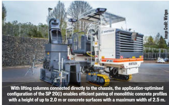
With lifting columns connected directly to the chassis, the application-optimised configuration of the SP 20(i) enables efficient paving of monolithic concrete profiles with a height of up to 2.0 m or concrete surfaces with a maximum width of 2.5 m.
