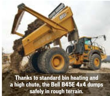
Thanks to standard bin heating and a high chute, the Bell B45E 4x4 dumps safely in rough terrain.
